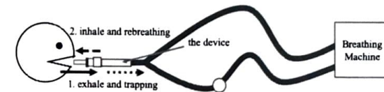
Moisture (and heat) from exhalation "trapped" by the device and then re-breathed on the next breath
